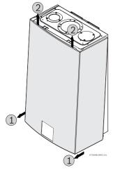
Fig. 4 Removing the front cover
